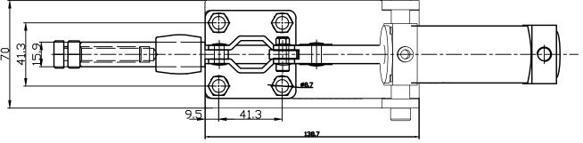
HOLDING CAPACITY:386Kg PLUNGER STROKE:23.6mm
